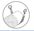
Prepare pipe end by de-scaling if required. Clean the pipe as required with water. Make sure that the pipe is clean from debris and defects that interfere with HYMAX GRIP's proper seal.
