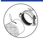
Mark pipe end to a minimum required stab depth as indicated on the product label. These marks indicate the required stab depth of the pipe on the HYMAX GRIP End Cap.
