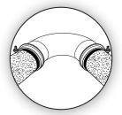
Position the elbow for installation. Place the elbow with top-facing bolts. Slide the coupling so that it covers the marks made in step 4. Make sure that the pipes are properly supported.
