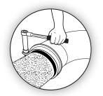
Tightening the end rings. Tighten the Elbow's bolts using a 3/4" socket wrench for 2"-3" couplings, a 7/8" socket wrench for 4"-12" couplings. Tighten the bolts evenly on each end ring in an alternating pattern to the torque mentioned on the label. Cross-tightening ensures that the gasket is evenly seated. When you finish, re-check the torque again. **DO NOT LUBRICATE BOLTS!**
