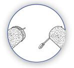
Measure both pipes' outer diameters and make sure the Elbow's size will fit the pipes properly on both sides.
