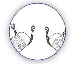
Prepare both pipe ends by descaling if required. Clean the pipes as required using water. Make sure that the pipe is clear from debris and defects that may interfere with the HYMAX Elbow's proper seal.
