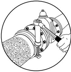
Tightening the end rings. Tighten the Flange Adaptor's bolts using a 15/16" socket wrench for 14"-24" Flange Adaptors, and a 1.5" socket wrench for 26"-60" Flange Adaptors. Tighten the bolts evenly on each end ring in an alternating pattern to the torque mentioned on the label. Cross-tightening ensures that the gasket is evenly seated. When you finish, re-check the torque again.
