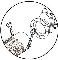
Prepare the pipe end. Clean and de-scale pipe end. Remove any debris or build up on the pipe end and clean the outer pipe surface with soapy water. Clean pipe end to a distance that is equal to the length of the center ring. Make sure there is no corrosion on the outer pipe end that could affect the gasket seal. Again, clean pipe end with water.
